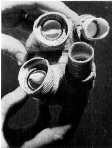
FIGURE 4 A polyurethane hemispherical artificial heart. (a) The molds and a polyurethane diaphragm and shell for one ventricle; (b) view of both ventricles after termination of implantation. Reproduced with permission of the Transactions of the American Society for Artificial Internal Organs (Ref. 27).
